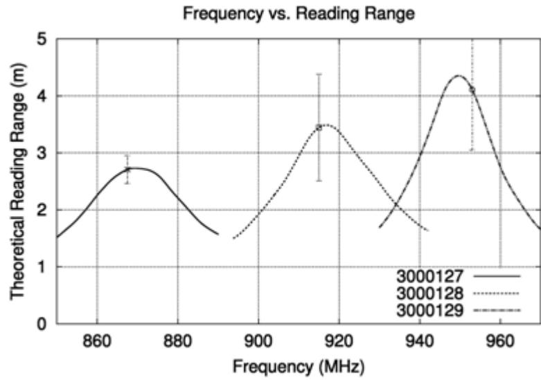
\* Read ranges are theoretical values that are calculated for non-reflective environment, in where antennas with optimum directivity are used with maximum allowed operating power according to ETSI EN 302 208 (2W ERP). Variation of 3σ from test batch marked in the picture. Note, tag performance in other frequency bands is not marked in the picture; tag will remain functional but the performance is low.
