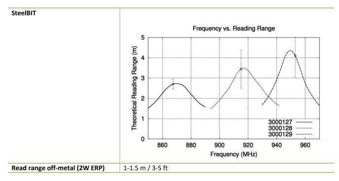
\* Read ranges are theoretical values that are calculated for non-reflective environment, in where antennas with optimum directivity are used with maximum allowed operating power according to ETSI EN 302 208 (2W ERP). Variation of 3 $\sigma$  from test batch marked in the picture. Note, tag performance in other frequency bands is not marked in the picture; tag will remain functional but the performance is low.
