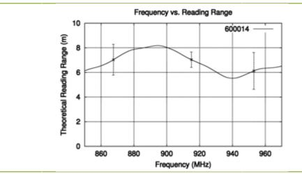
Presented reading ranges are calculated values in non-reflective environment, in where antennas with optimum directivity are used with maximum allowed operating power: EU 865-868 MHz (2W ERP), US 902-928 MHz (4W EIRP), and JPN 952-954MHz (4W EIRP).
