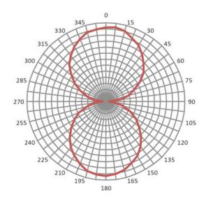
Angular Sensitivity (Relative Read Range vs. Orientation)
