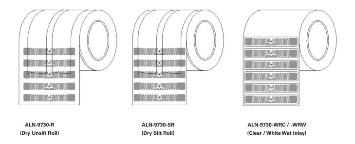
Standard Alien Inlay rolls unwind with metal antenna side facing outward, with respect to the core.
